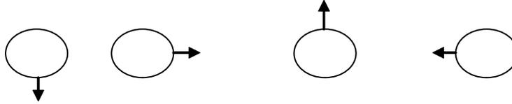
**g. Off-page connectors:** This connector represents a break in the path of flowchart which is too large to fit on a single page. It is similar to on-page connector. The connector symbol marks where the algorithm ends on the first page and where it continues on the second.
